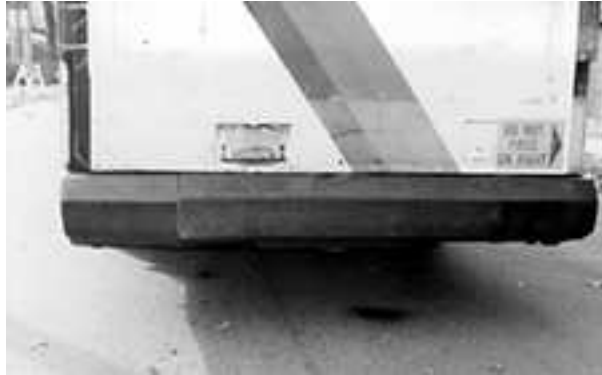
Figure 5 - Cumulative Damage to Flexible Bus
